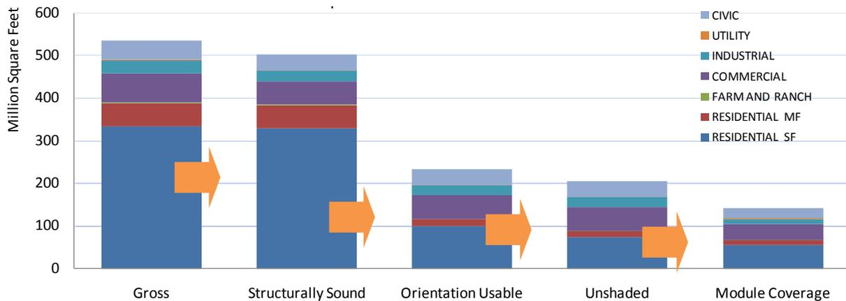
**Figure 3. Rooftop Area Screening Details: Area Suitable for PV Installation, by Property Type**
